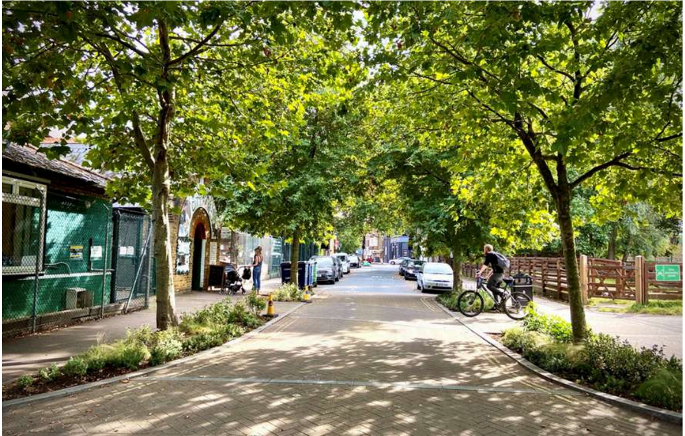
Street trees limit lane widths to ensure safe traffic speeds in London, UK. Photo: Tree for Streets.
