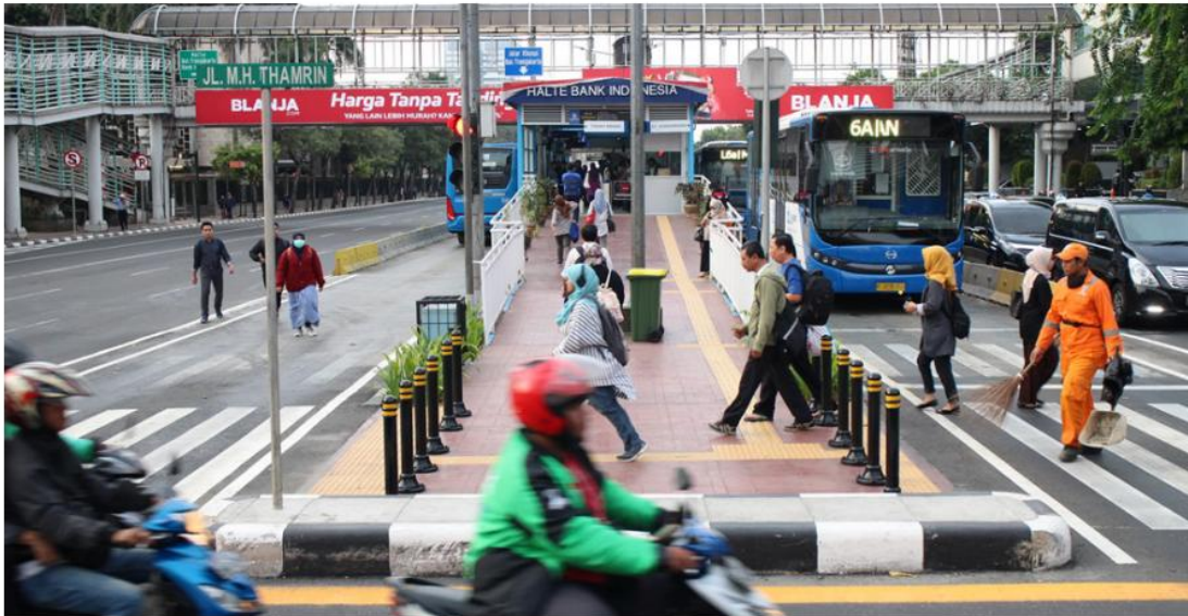
Figure 54. BRT station at-grade crossing
